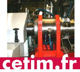
Cetim disposes of test benches to perform the tests detailed in the document Pr EN 16752 « Centrifugal pumps – Test procedure for seal packing » : an ESA – FSA type test bench, specifically for packings and a high performance test bench
